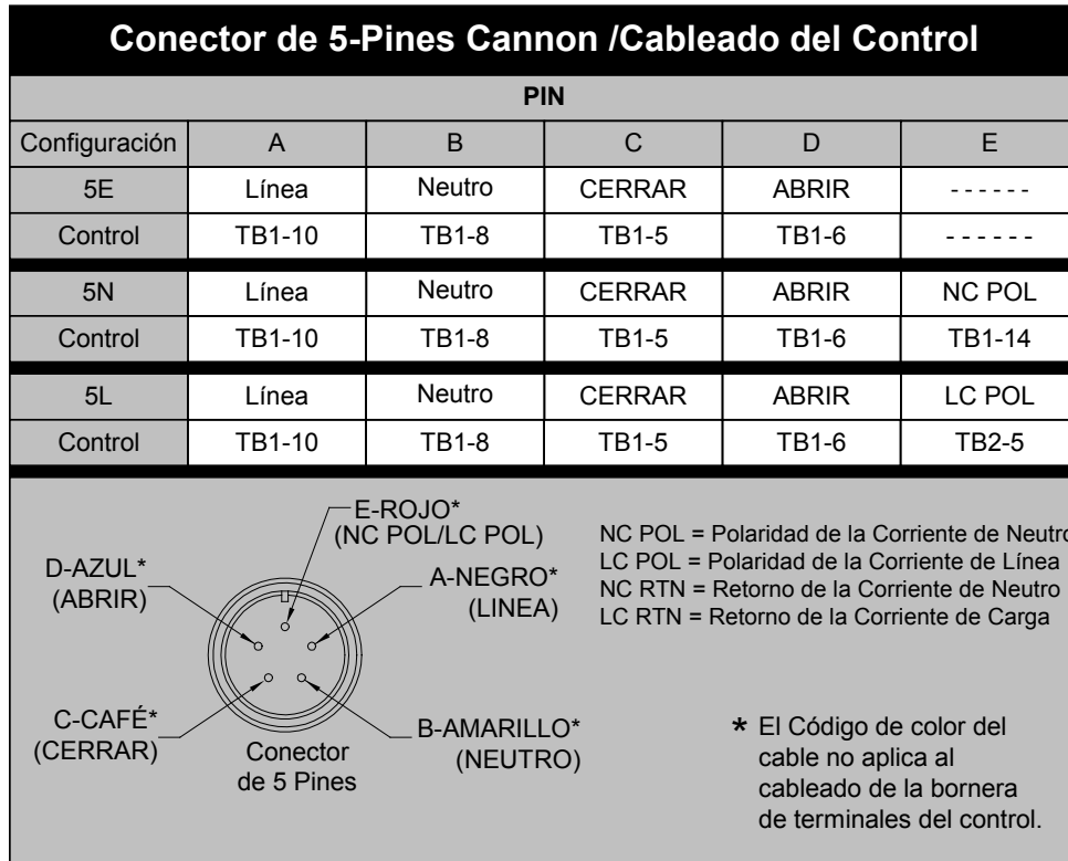
Figura 13 Conector de 5-Pines Cannon/Cableado del Control
