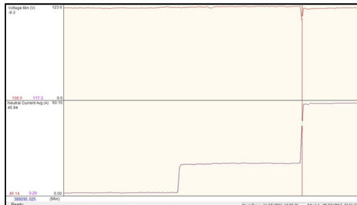
Figure 2: Datalog showing increased neutral current when fuse failed
